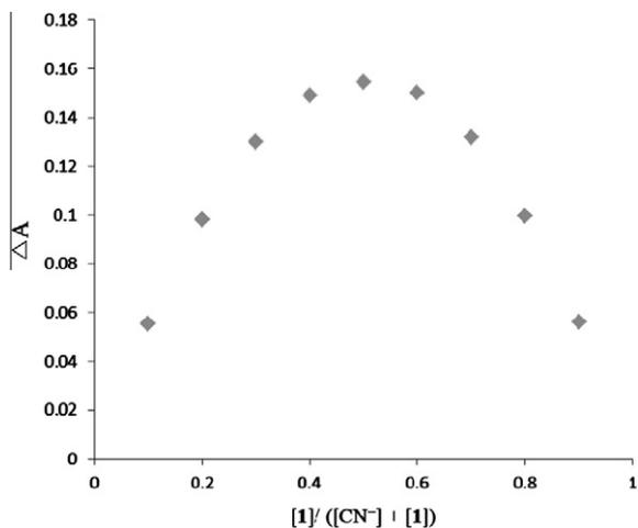
Figure 4. Job plots of receptor **1** and cyanide in ethanol.
