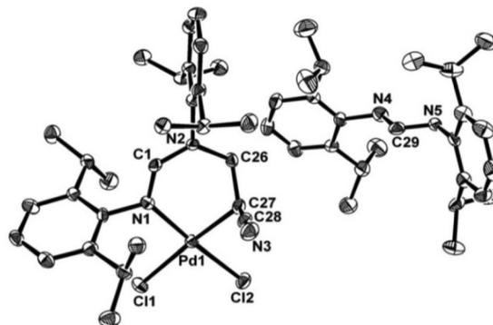
Fig. 3 ORTEP diagram showing 50% probability thermal ellipsoids and selected atom labels for 10. Hydrogen atoms and one solvent DCM molecule have been omitted for clarity.
