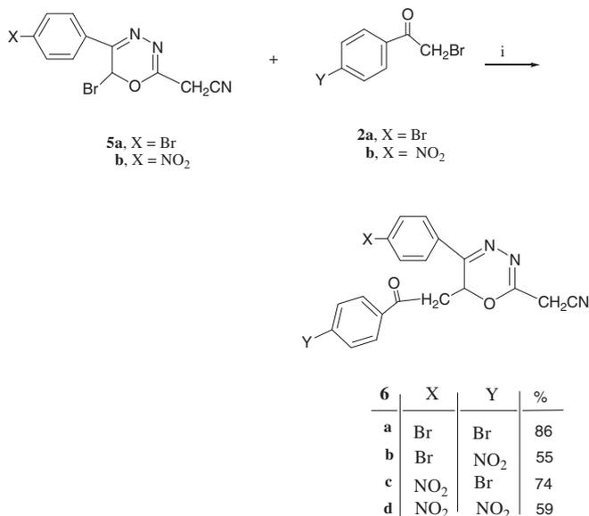
**Scheme 2.** Reagents and conditions: (i) Pd(PPh<sub>3</sub>)<sub>4</sub>, toluene, MeOH, Na<sub>2</sub>CO<sub>3</sub>, reflux 15 h at 80 °C, column chromatography (SiO<sub>2</sub>, hexan, EtOAc 9:1, then 4:1).
