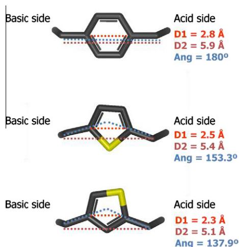
Figure 2. Geometric parameters of phenyl and thiophenes central cores.
