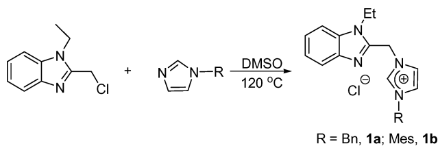
Scheme 1 Synthesis of ligand precursor [\text{HL}]^+\text{Cl}^- .
