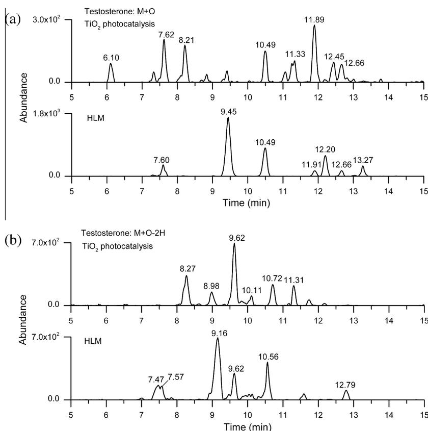
**Fig. 3.** Extracted ion chromatograms of (a)  $m/z$  305.2117 and (b)  $m/z$  303.1960 corresponding to  $M+O$  and  $M+O-2H$  reaction products of testosterone, respectively. Peaks observed at the same retention time and with matching MS/MS spectra in  $\text{TiO}_2$  photocatalysis and HLM reactions were considered identical compounds.
