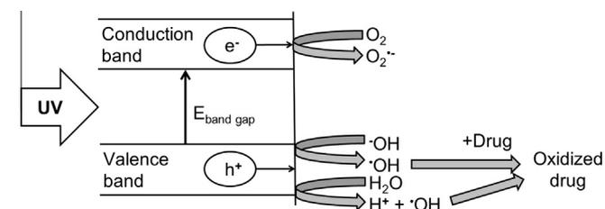
**Fig. 1.** The principle of  $\text{TiO}_2$  photocatalysis. Modified from (Bhatkhande et al., 2002). See Fujishima et al. (2008) and Zhang et al. (2012) for more detailed descriptions of the  $\text{TiO}_2$  photocatalysis mechanism.
