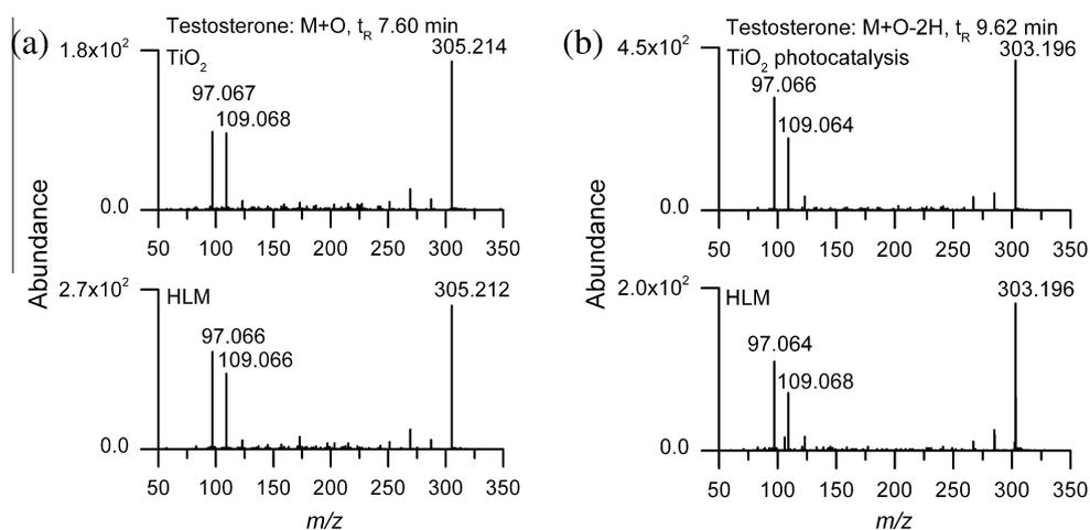
**Fig. 5.** Examples of correlation of MS/MS spectra (CE 20 V) in  $\text{TiO}_2$  photocatalysis and HLM reactions. (a) MS/MS spectra of M+O ( $m/z$  305.2117,  $t_R$  7.60 min) and (b) MS/MS spectra of M+O-2H ( $m/z$  303.1960,  $t_R$  9.62 min) reaction product of testosterone.
