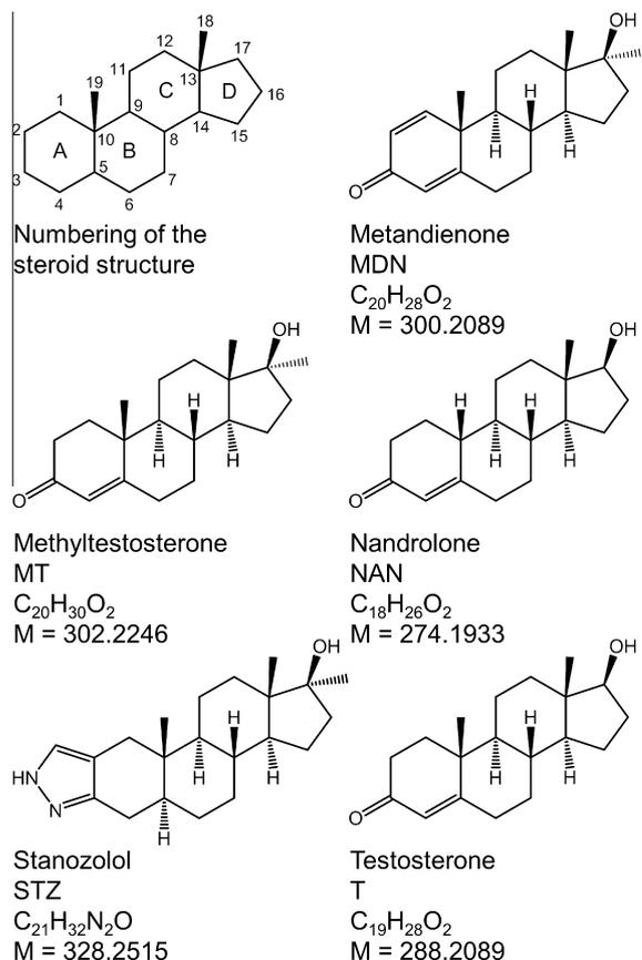
**Fig. 2.** Molecular structures, names, abbreviations, molecular formulas and mono-isotopic masses of the test compounds used in this study. Top-left figure represents the numbering of the different carbon atoms in the steroid structure.
