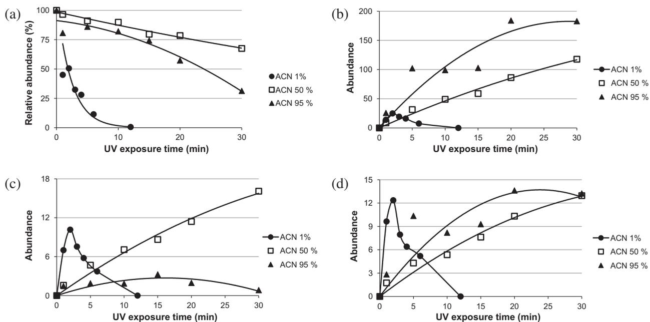
**Fig. 4.** Effect of acetonitrile concentration on degradation of testosterone and formation of selected photocatalytic reaction products of testosterone. (a) Degradation of testosterone ( $m/z$  289.22,  $t_R$  3.55 min), (b) formation of an M-2H product ( $m/z$  287.20,  $t_R$  3.34 min), (c) formation of an M+O product ( $m/z$  305.21,  $t_R$  2.99 min), and (d) formation of an M+O-2H reaction product ( $m/z$  303.20,  $t_R$  2.67 min) of testosterone.
