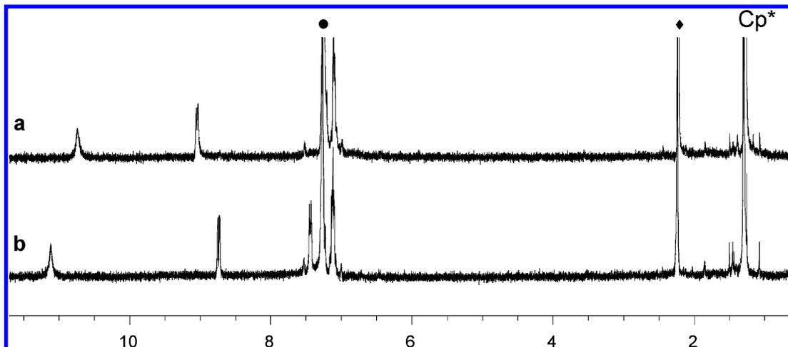
**Figure 2.**  $^1\text{H}$  NMR spectra of one sample of  $[\text{Cp}^*\text{RuCl}(\mu\text{-NHPh})]_2$  in  $\text{C}_6\text{D}_6$  (●) and with a  $\text{C}_6\text{Me}_6$  internal standard (◆): (a) the initial  $C_{2v}$  isomer **1b**; (b) the  $C_i$  isomer **1a** after isomerization.
