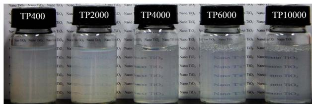
Fig. 1 Photographs of the PEG-capped TiO<sub>2</sub> NPs aqueous solutions.
