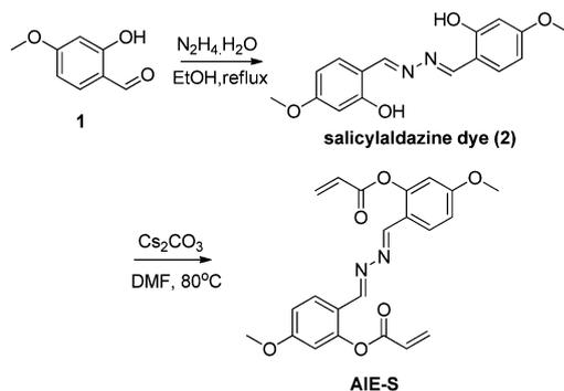
Scheme 2 Synthetic route for the probe AIE-S.
