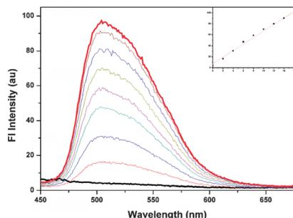
Fig. 4 Fluorescence spectra of 10  $\mu\text{M}$  **AIE-S** in the presence of different amounts of Cys (from 0 to 16  $\mu\text{M}$ ) in PBS buffer (10 mM, pH = 7.4, 1% DMSO),  $\lambda_{\text{ex}} = 340$  nm. Inset: The fluorescence intensity at 505 nm as a function of Cys concentration.
