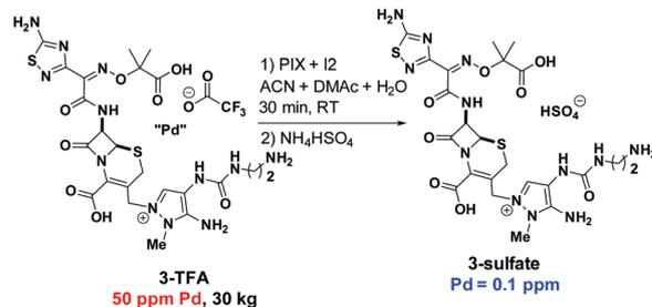
**Scheme 5** Zerbaxa ceftolozane palladium removal with PIX on pilot plant scale.
