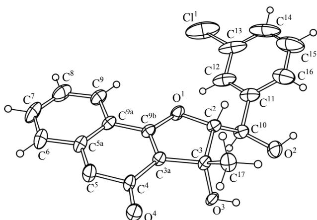
**Fig. 1.** Structure of the molecule of 2-[(3-chlorophenyl)(hydroxy)methyl]-3-hydroxy-3-methyl-2,3-dihydro-4*H*-furo[3,2-*c*]chromen-4-one (**VII**, diastereoisomer **A**) according to the X-ray diffraction data. Non-hydrogen atoms are shown as thermal vibration ellipsoids with a probability of 30%.
