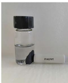
**FIGURE 8** The recycling runs for Ni/CNT catalyst in the catalytic transfer hydrogenation and magnetic recovery of Ni/CNT catalyst
