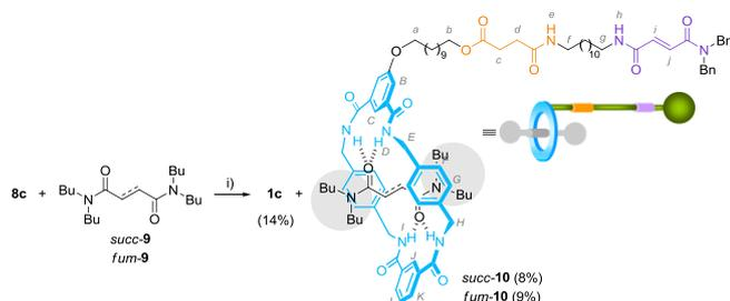
**Scheme 3** Competitive coupling of the diamine **8c** with isophthaloyl chloride in the presence of single binding-site threads: formation of the [1]rotaxane **1c** using an intramolecular template *versus* the formation of [2]rotaxanes **10** using the intermolecular dicarboxamide-based templates **9**. Reagent and conditions: i) isophthaloyl chloride, Et<sub>3</sub>N, CHCl<sub>3</sub>, 25 °C.
