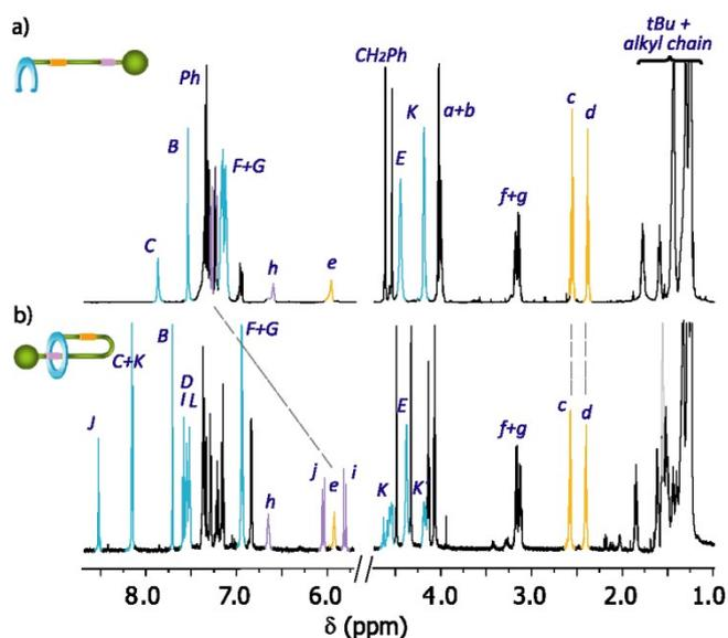
**Fig. 2** Partial  $^1\text{H}$  NMR spectra (600 MHz,  $\text{CD}_2\text{Cl}_2$ , 298 K) of (a) precursor **7c** and (b) [1]rotaxane **1c**. The assignments correspond to the lettering shown in Schemes 1 and 2.
