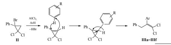
The products of the reaction of aromatic compounds **Ia–Id** with reagent **II** were isolated by vacuum distillation as individual compounds (**IIIa**, **IIId**) or as mixtures of isomers (**IIIb** + **IIIc**, **IIIe** + **IIIf**). Their structure and the ratio of *ortho-* and *para-*isomers in the mixture were determined by the <sup>1</sup>H and <sup>13</sup>C NMR spectroscopy, GC-MS method.
