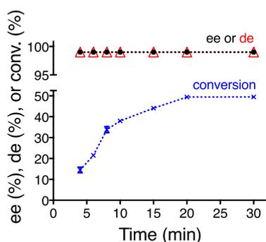
**Fig. 2.** Kinetic resolution of *rac*-1-phenylallyl alcohol by HhMo. The conversion (cross, X), ee (filled circle, ●), and de (blank triangle, △) were determined by chiral HPLC. Standard deviations of triplicates are represented by error bars.
