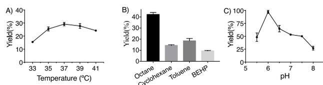
**Fig. 1.** The effects of temperature, co-solvent, and pH on the HhMo-catalyzed epoxidation. Whole *E. coli* cells expressing HhMo and PsStyB were used to convert allylbenzene, and the yields of the product were measured by GC. Standard deviations of triplicates are represented by error bars.
