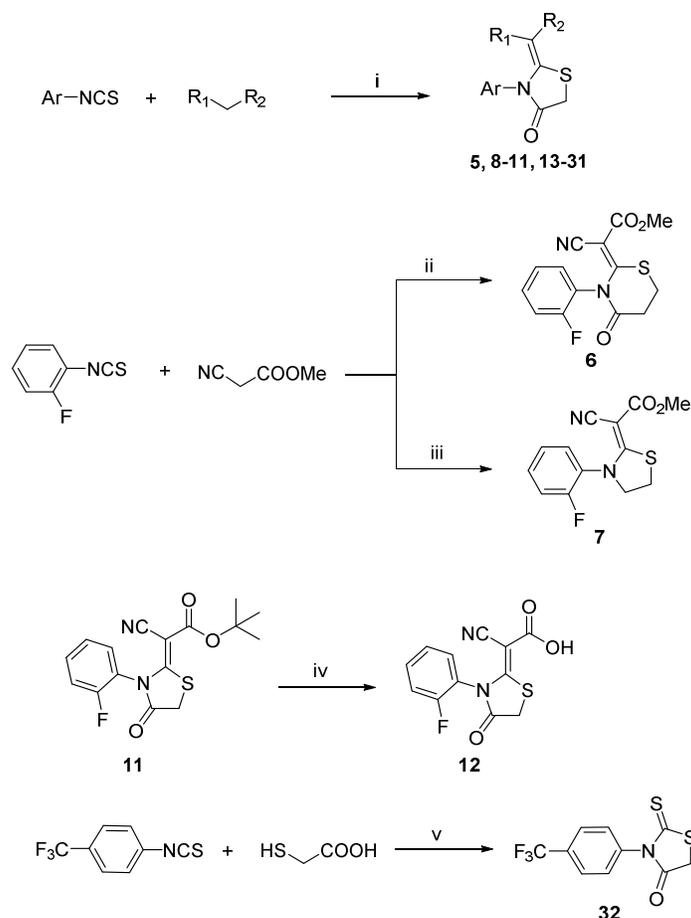
**Scheme 2.** Synthesis of compounds **5-32**. (i) KOH, DMF, r.t. 15-30 min;  $\text{ClCH}_2\text{COCl}$ ,  $0\text{ }^\circ\text{C}$ ; r.t., 12 h, 68%-80%. (ii) KOH, DMF, r.t. 15 min;  $\text{BrCH}_2\text{CH}_2\text{COCl}$ ,  $0\text{ }^\circ\text{C}$ ; r.t., 12 h, 60%. (iii) KOH, DMF, r.t. 15 min;  $\text{BrCH}_2\text{CH}_2\text{Br}$ ,  $0\text{ }^\circ\text{C}$ ; r.t., 12 h, 48%. (iv) TFA, DCM, r.t. 85%. (v) TEA, dioxane, reflux, 65%.
