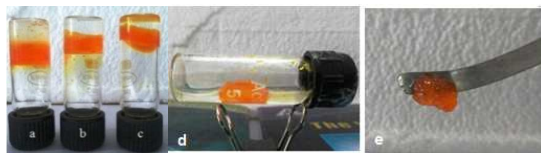
Figure 12. Phase selective gelation of 9a (0.02 g) in equiv. volume of water with aromatic solvents such as (a) xylene (b) toluene (c) benzene. (d) Tilted vial after phase selective gelation of xylene showing gel stability in water (e) xylene gel scooped out with a spatula
