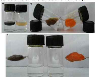
Figure 14. Real-time example of oil-spill remediation by phase selective gelation of petrol and crude oil using 9a from a biphasic mixture of petrol/crude oil and water. (a) vial showing mixture of crude oil (2 mL, left) and petrol (2 mL right) with water (5 mL) (b) tilted vials showing phase selective gelation of crude oil (left) and petrol (right) (c) crude oil gel (left)
