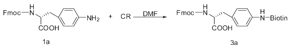
Scheme 1 Synthesis of Fmoc-D-Aph(Bio) under different conditions. CR represented coupling reagent(s), either biotin hydroxysuccinimide ester or biotin with a coupling reagent.
