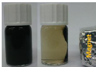
Fig. 4 Separation of the dispersed catalyst \text{Fe}_3\text{O}_4/\text{tart} -NPs in acetonitrile (left) by using an external magnet (right).
