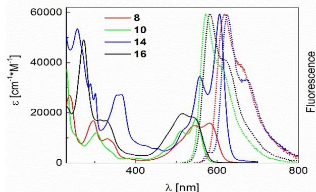
Figure 1. Absorption and fluorescence spectra for **8**, **10**, **14** and **16** in DCM.
