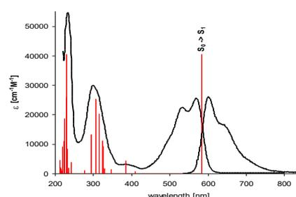
Figure 2. Experimental absorption and fluorescence spectra of **2** in DCM. Calculated transition energies from the ground  $S_0$  to the electronically excited states are given by vertical solid lines with the heights proportional to the oscillator strength of the transition (see Table S3 for the details). Vibronic structure is smoothed by low frequency vibrations (for interpretation see Fig. S6).
