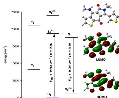
Figure 3. Energy diagram with the transition energies for absorption from the ground  $S_0$  state to the  $S_1^{\text{FC}}$  and fluorescence from the relaxed  $S_1$  state to  $S_0^{\text{FC}}$  for **2**. On the right - the orbitals HOMO and LUMO of **2**. Electronic configuration HOMO  $\rightarrow$  LUMO describes the transition  $S_0 \rightarrow S_1$ .
