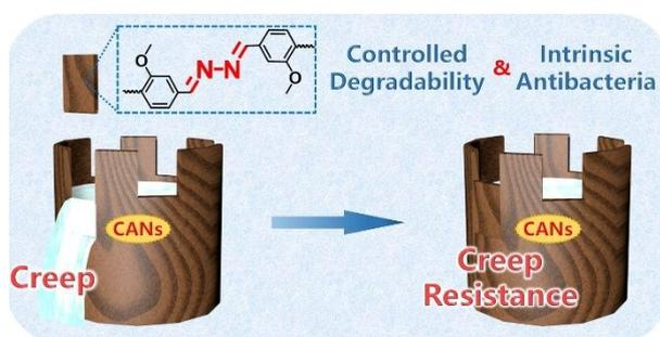
This work highlights the exploitation of dihydrazone motif to build antibacterial covalent adaptable networks with no creep at  $\sim 105$  °C.
