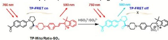
**Scheme 1** Response Mechanism of TP-Mito/Ratio-SO<sub>2</sub> toward SO<sub>2</sub> Derivatives
