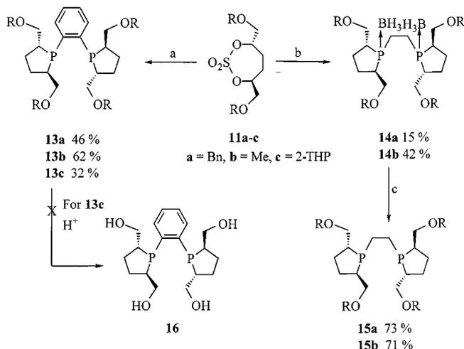
Scheme 4. Reagents and conditions: a: 1. BuLi, THF, -78 °C to room temp., 2 h; 2. 1,2-(H<sub>2</sub>P)<sub>2</sub>C<sub>6</sub>H<sub>4</sub>, -78 °C to room temp.; 3. BuLi, -78 °C to room temp., 12 h; b: 1. BuLi, THF, -78 °C to room temp., 2 h; 2. H<sub>2</sub>P-C<sub>2</sub>H<sub>4</sub>-PH<sub>2</sub>, -78 °C to room temp.; 3. BuLi, -78 °C to room temp., 12 h; 4. BH<sub>3</sub>-THF, -10 °C to room temp., 2 h; c: DABCO, toluene, 40 °C
