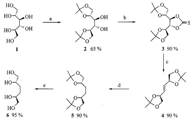
Scheme 1. Reagents and conditions: a: acetone, ZnCl<sub>2</sub>, 25 °C, 2 h; b: S=CCl<sub>2</sub>, DMAP, 0 °C, 1 h; c: P(OEt)<sub>3</sub>, 160 °C, 20 h; d: H<sub>2</sub>, Rh/Al<sub>2</sub>O<sub>3</sub>, THF, room temp. or H<sub>2</sub>, Pt/C, MeOH, room temp.; e: 2 N HCl, 80 °C, 2 h
