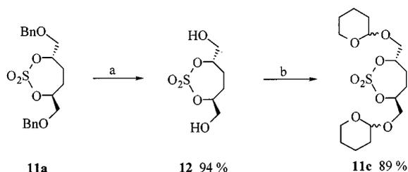
Scheme 3. Reagents and conditions: a: 1 bar H<sub>2</sub>, Pd/C, MeOH, room temp.; b: 3,4-dihydro-2H-pyran, PPTS, CH<sub>2</sub>Cl<sub>2</sub>, room temp., 2 h
