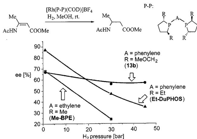
Figure 3. Dependency of the *ee* upon the H<sub>2</sub> pressure with [Rh(COD)(P-P)]BF<sub>4</sub> (P-P: **13b**, Et-DuPHOS, Me-DuPHOS) in the hydrogenation of methyl (*Z*)-3-(acetyl-amino)butenoate
