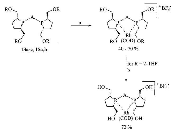
Scheme 5. Reagents and conditions: a: [Rh(COD)<sub>2</sub>]BF<sub>4</sub>, THF, 0 °C to room temp., 1 h; b: aq. HBF<sub>4</sub>, MeOH, room temp., 24 h
