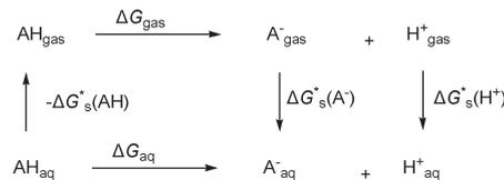
**Scheme 3** Thermodynamic cycle used in the calculation of the *pK*<sub>a</sub> of the amino acid ionic liquids.
