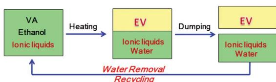
Fig. 1 The esterification for EV catalyzed by amino acid ionic liquids.
