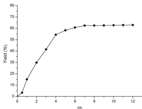
**Fig. 2** The esterification to produce EV after different reaction times at room temperature (reaction conditions: catalyst = ProHSO<sub>4</sub> (50 mol%, based on VA), VA/ethanol (molar ratio) = 1; conversion and selectivity of EV determined by GC analysis).
