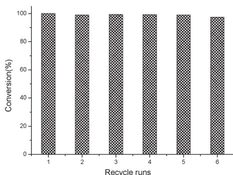
**Fig. 3** Reaction recycling of the esterification for EV production over ProHSO<sub>4</sub> catalyst.
