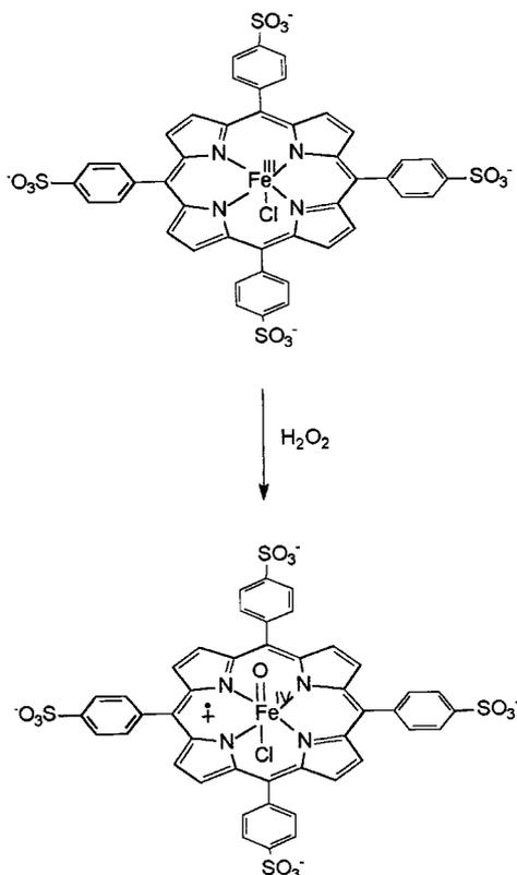
Scheme 3. Formation of the active oxidant by reaction of FeTPPSCl with  $H_2O_2$
