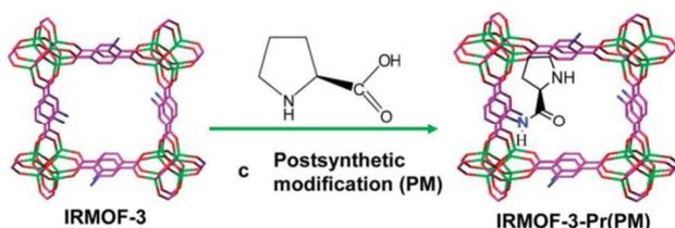
Fig. 1. Synthesis of IRMOF-3-Pr(PM). Reprinted with permission from ref. 1
