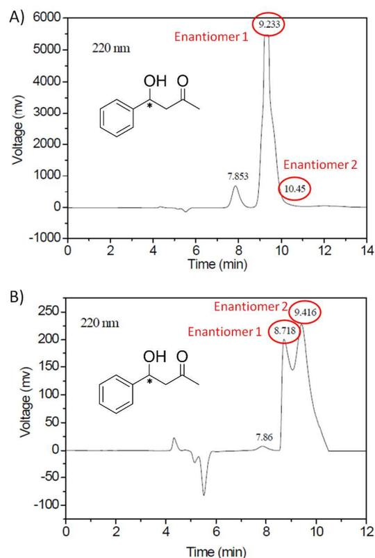
**Fig. 3.** HPLC trace of IRMOF-3-Pr(PM)-catalyzed aldol reaction products (A) when catalysis is performed at room temperature showing 93% e.e. and (B) when catalysis is performed at 40°C showing 33% e.e. Both chromatograms are recorded for the same aldol compounds under the same analytical conditions. Reprinted with permission from ref. 1
