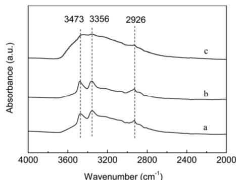
**Fig. 2.** Infrared spectra of IRMOF-3 (a) and IRMOF-3-Pr(PM) (c) samples. Reprinted with permission from ref. 1
