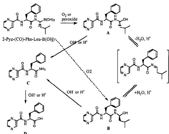
**Scheme 1.** Proposed mechanism for the degradation of 2-Pyz-(CO)-Phe-Leu-B(OH)<sub>2</sub> under oxidative, acidic, and alkaline conditions.
