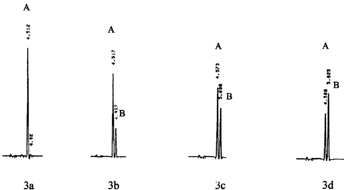
**Figure 3.** HPLC chromatogram of transformation of degradant **A** (1.1 mM) to **B** under acidic conditions. Figures a, b, c, and d correspond to times of transformation for 0, 20, 30, and 128 min, respectively, at pH 2.0 and room temperature.
