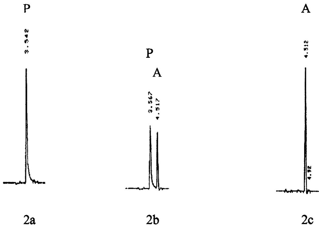
**Figure 2.** HPLC chromatograms of the reaction of 2-Pyz-(CO)-Phe-Leu-B(OH) $_2$  (1.1 mM) with H $_2$ O $_2$  (15.7 mM) in H $_2$ O at room temperature. Figures a, b, and c correspond to reaction times of 0, 15, and 60 min, respectively, and **P** and **A** represent the parent compound and degradant **A**, respectively.
