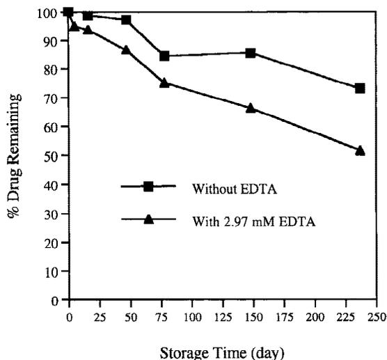
**Figure 5.** Plot showing the effect of EDTA on the stability of 2-Pyz-(CO)-Phe-Leu-B(OH)<sub>2</sub> (1.3 mM) at 25 °C. The solvent was 2% EtOH and 98% normal saline (pH 6.9) with and without 2.97 mM EDTA.
