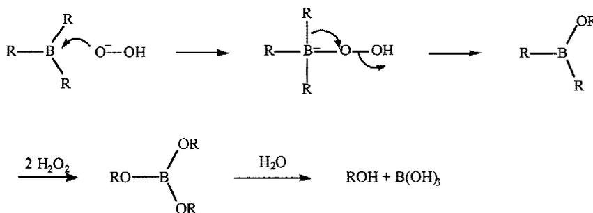
**Scheme 2.** The mechanism for oxidation of alkyl boranes by hydrogen peroxide.<sup>8</sup>
