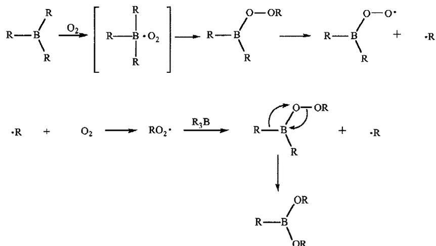
**Scheme 3.** The mechanism for oxidation of alkyl boranes by oxygen.<sup>9-11</sup>
