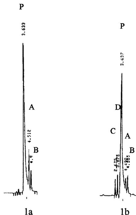
**Figure 1.** HPLC chromatograms illustrating degradation of 2-Pyz-(CO)-Phe-Leu-B(OH)<sub>2</sub> in solvents of (a) PEG300:EtOH:H<sub>2</sub>O (40:10:50) and (b) EtOH:normal saline (2:98) (pH 2.83); **P**, **A**, **B**, **C**, and **D** represent the parent compound and degradants **A**, **B**, **C**, and **D** respectively.
