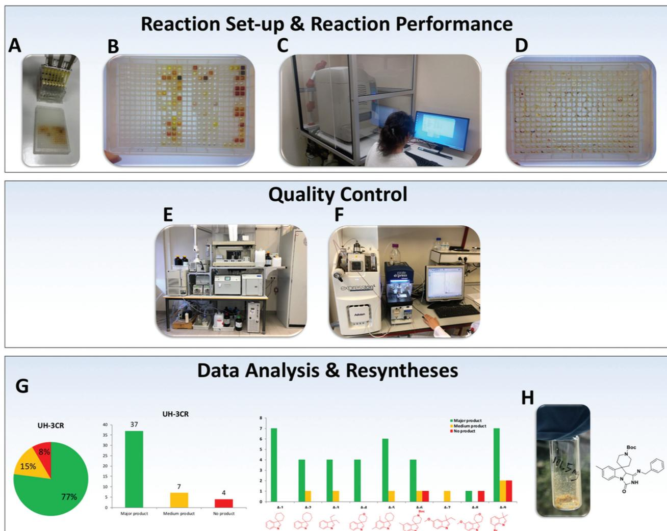
**Fig. 6** Workflow of automated and accelerated ADE-enabled syntheses. Above: Preparation of stock solutions of building blocks (A) and transfer into 386-well source plates (B); ADE workplace with an ECHO555 in a chemical hood and an external remote computer control (C); a 384-well destination plate (D). Middle: Quality control with SFC-MS (E) and TLC-UV-MS (F). Bottom: Data analysis (G) and resynthesis of compounds on a 0.5 mmol scale (H).
