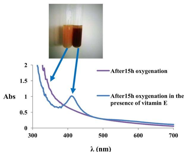
**Fig. 3.** Benzaldehyde oxidation process in the presence of vitamin E (orange tube) and in the absence of vitamin E (dark red)
