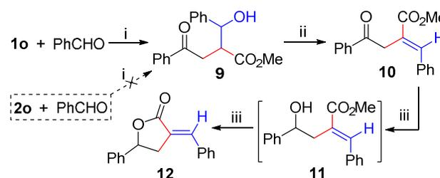
**Scheme 7.** Tandem allylic isomerization-Aldol reaction for the synthesis of (*E*)- $\alpha$ -alkenyl- $\gamma$ -butyrolactone. i: **1**: Mg(OMe)<sub>2</sub>: TMEDA: PhCHO = 1: 0.67: 0.5: 1, 89%. ii: TFA (30 equ.), CH<sub>2</sub>Cl<sub>2</sub>, 98%. iii: a) NaBH<sub>4</sub> (3 equ.), MeOH, then b) HCl (1M) in one-pot, 70% for the two steps.
