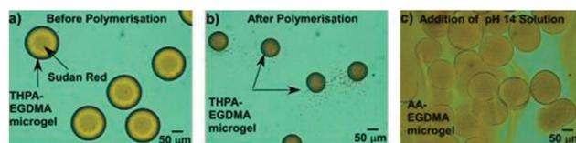
Fig. 6 (a) 50:4 THPA-EGDMA microgels with hydrophobic Sudan I dye encapsulated during droplet generation. (b) 50:4 THPA-EGDMA droplets after polymerisation (pH = 7). (c) Sudan I dye release from 50:4 AA-EGDMA microgels in pH 14 solution.
