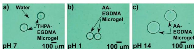
Fig. 4 THPA-EGDMA (50:4 molar ratio) microgels (a) before hydrolysis at pH 7, (b) after hydrolysis (forming AA-EGDMA microgels) at pH 1, and (c) at pH 14.
