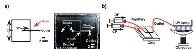
Fig. 2 (a) Layout and photograph of the flow focusing chip employed for microgel precursor droplet formation. The design featured a central channel for the oil based DP, containing the reagents, and outer channels for the CP, which merged into a 5 mm long outlet channel. (b) Experimental setup for on-chip droplet generation and collection of the droplets onto a slide or dish for UV initiated photopolymerisation.
