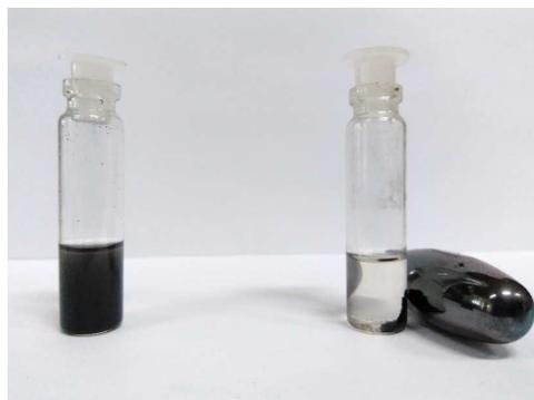
**Figure 3.** Separation of catalyst Glu-Fe<sub>3</sub>O<sub>4</sub>-SO<sub>3</sub>H using external magnetic field.
