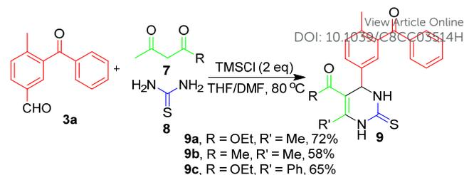
**Scheme 3** Application of the benzaldehydes in Biginelli reaction
