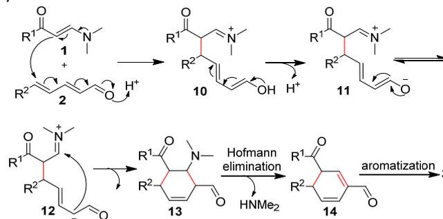
**Scheme 4** The proposed mechanism for the benzannulation-based synthesis of benzaldehydes
