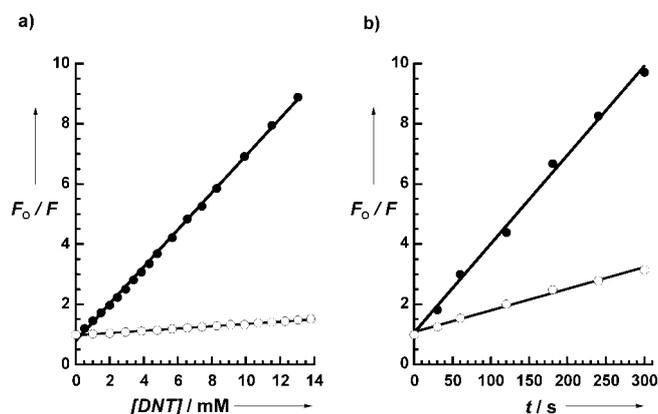
Figure 4. Stern–Volmer plots of **3** in a nonaggregated form (○) and an aggregated form (●) in solutions at OD = 0.09 (a). Stern–Volmer plot of **2** (○) and **3** (●) in films of OD = 0.03 upon exposure to TNT vapors (b).
