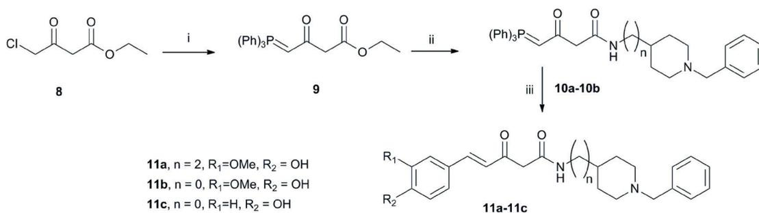
**Scheme 3** Synthesis of **11a–11c**. Reagents and conditions: (i) Ph<sub>3</sub>P, toluene, 50 °C, 24 h; (ii) xylene, reflux; (iii) NaH, THF, 40 °C, 3 h, rt, overnight.
