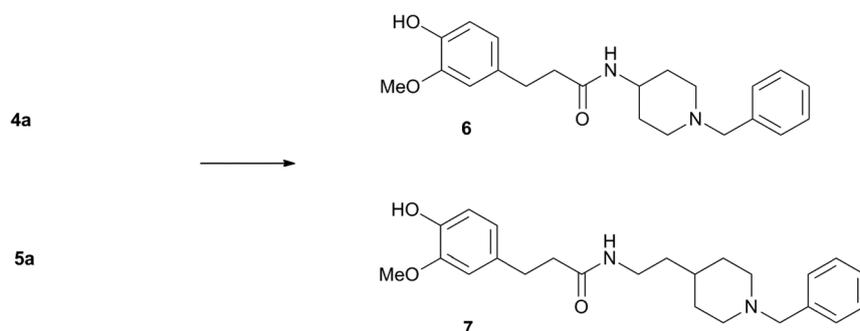
**Scheme 2** Synthesis of **6** and **7**. Reagents and conditions: H<sub>2</sub>, Pd/C, MeOH, rt, 8 h.
