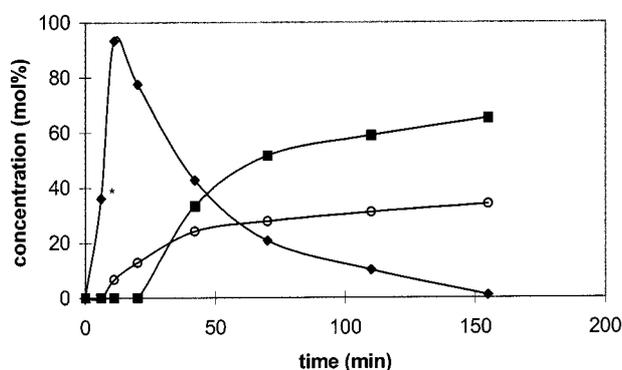
Figure 5. Concentrations of benzylamine (■), dibenzylamine (○), and dibenzylimine (◆) during the reductive amination of benzaldehyde; 80 mL of 2 M NH<sub>3</sub>/MeOH, 17 mg Pd/SX1GNS150, 1 g of benzaldehyde, 90 °C and 40 bar H<sub>2</sub>. \*At this point, the mass balance was < 100%, most probably due to the formation of hydrobenzamide when the sample was cooled down. This compound was not analyzed, but could be precipitated on the catalyst
