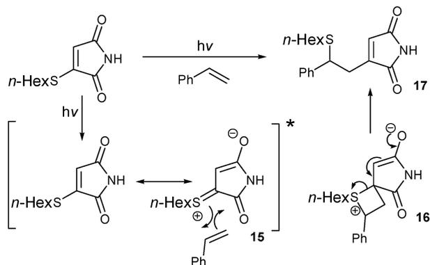
**Scheme 2** Insertion of styrene in to the C–S bond.
