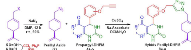
Scheme 2. Synthesis of Perillyl Azide and the Cu(I) catalyzed Huisgen reaction
