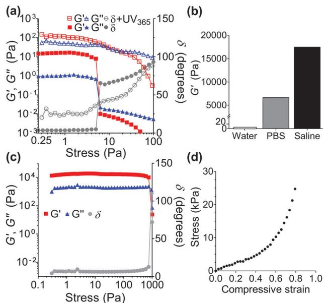
Fig. 5 Oscillatory shear testing of hydrogels prepared from **A** at 10 mM showing stress sweeps of gels in pure water for both non-irradiated and irradiated hydrogels (a); summarized elastic storage moduli ( $G'$ ) for non-irradiated hydrogels prepared in various aqueous solutions (*i.e.*, water, PBS, and saline) (b); non-irradiated hydrogels in saline (0.9% NaCl) (c); and compressive properties of non-irradiated hydrogels prepared in saline (d).
