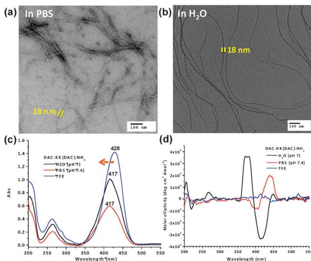
Fig. 2 TEM images of self-assembled dipeptide **A** in (a) PBS (pH 7.4) and (b) water (pH 7.0). (Carbon-coated copper grid, 2 wt% uranyl acetate as negative stain) (c) UV-vis spectra and (d) CD spectra of **A** in H<sub>2</sub>O, PBS and TFE. All solutions were prepared at 10 mM and freshly diluted to 0.25 mM after 1 day aging.
