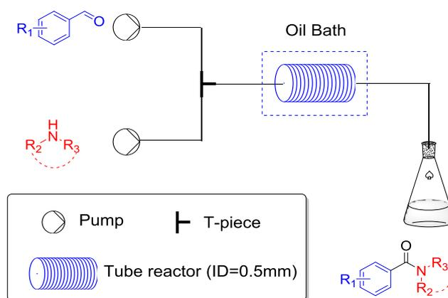
**Figure 1** Continuous flow system
