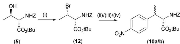
**Scheme 5** Reagents and conditions: (i) CBr<sub>4</sub>/PPh<sub>3</sub>, toluene, rt 5 h. (ii) Zn\*, DMF. (iii) bromide **5** in DMF, 1 h 35 °C. (iv) 4-NO<sub>2</sub>-C<sub>6</sub>H<sub>4</sub>I (1.33 eq.), Pd<sub>2</sub>(dba)<sub>3</sub> (2.5 mol%), P(*o*-MeC<sub>6</sub>H<sub>4</sub>)<sub>3</sub> (10 mol%), room temp., 3 h.
