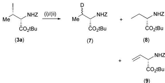
Scheme 3 Reagents and conditions: (i) Zn\* (prepared from Zn dust using 1,2-dibromoethane followed by Me<sub>3</sub>SiCl in DMF). (ii) Iodide **3a** in DMF 2 min then 2 eq. CH<sub>3</sub>COOD.
