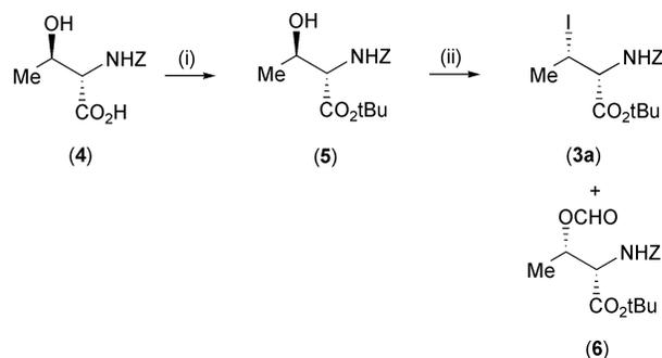
**Scheme 1** Reagents and conditions: i. *t*BuBr, benzyltriethylammonium chloride (BTEAC), K<sub>2</sub>CO<sub>3</sub>, DMA, 55 °C, 48 h. ii. 2 eq. Me(PhO)<sub>3</sub>P<sup>+</sup>I<sup>-</sup>, DMF, rt, 4 h.
