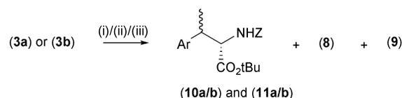
Scheme 4 Reagents and conditions: (i) Zn\* in DMF. (ii) iodide **3a** or **3b** in DMF, 2 min. (iii) ArI (1.33 eq.), Pd<sub>2</sub>(dba)<sub>3</sub> (2.5 mol%), P(*o*-MeC<sub>6</sub>H<sub>4</sub>)<sub>3</sub> (10 mol%), room temp., 3 h.
