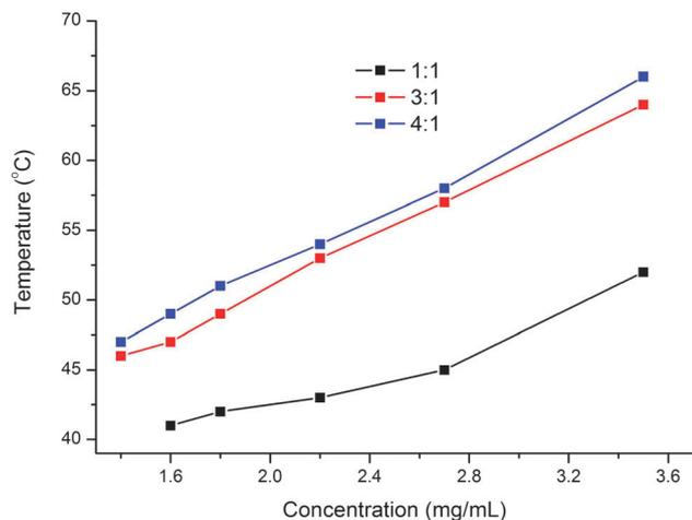
Fig. 6  $T_{\text{gel}}$ s of cyclohexane gels of **C12Ph**/**PDNA** vs. concentration.
