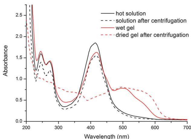
Fig. 4 UV-vis spectra of the mixture of **PDNA** and **C12Ph** in a 1 : 1 ratio in hot solution and gel, and the solution and dried gel after centrifugation.
