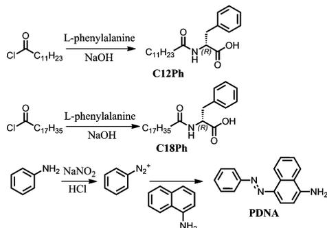
Scheme 1 Synthesis routes of **C12Ph**, **C18Ph**, and **PDNA**.
