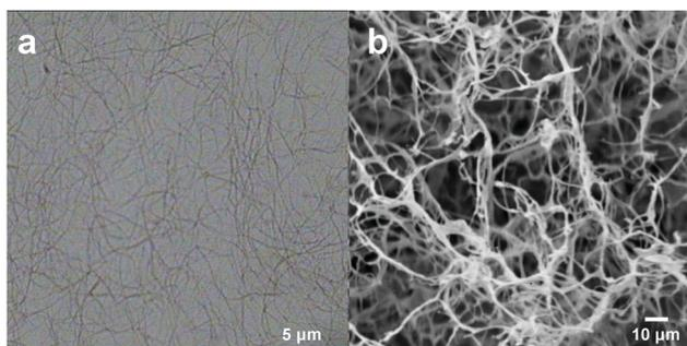
Fig. 2 (a) Optical microscopy images and (b) SEM images of the cyclohexane gel formed by **C12Ph** and **PDNA** (1 : 1).
