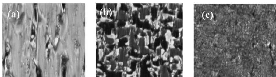
Fig. 9 Photomicrographs of (a) fan-shaped texture of the SmA phase (150 °C), (b) broken fan-shaped texture of the SmC phase (145 °C) and (c) non-specific texture of the SmCP phase (125 °C) observed for BC3-22 .
