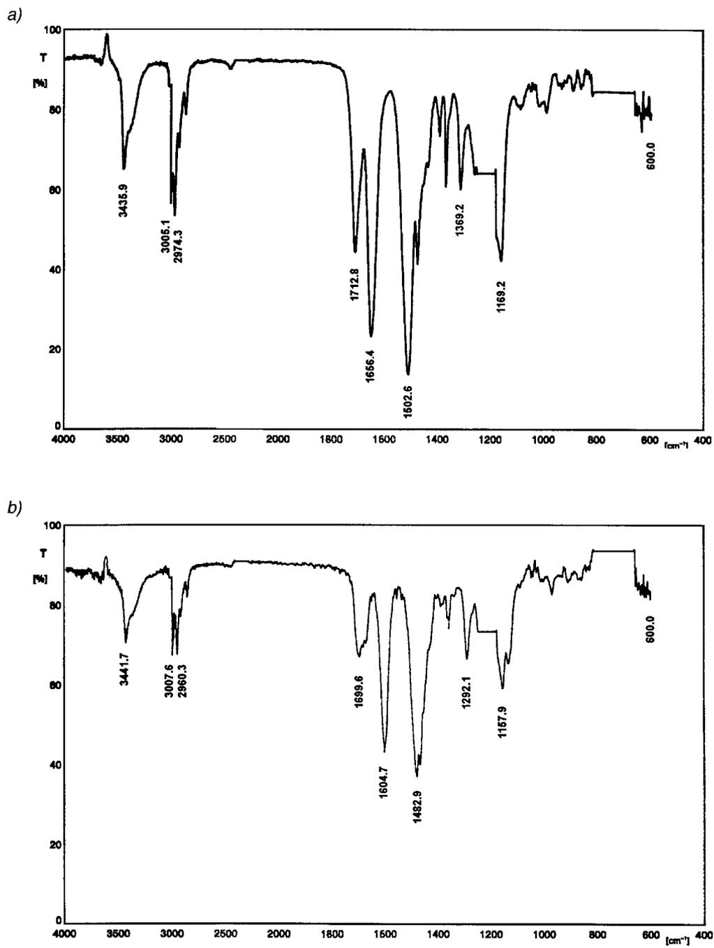
Fig. 4. IR Spectra of a) the unlabeled hexapeptide **2a** and b) the  $^{13}\text{C},^{15}\text{N}$ -labeled hexapeptide **2a\***. The spectra were measured in  $\text{CHCl}_3$  (concentration: 10 mg in 1 ml  $\text{CHCl}_3$ ).
