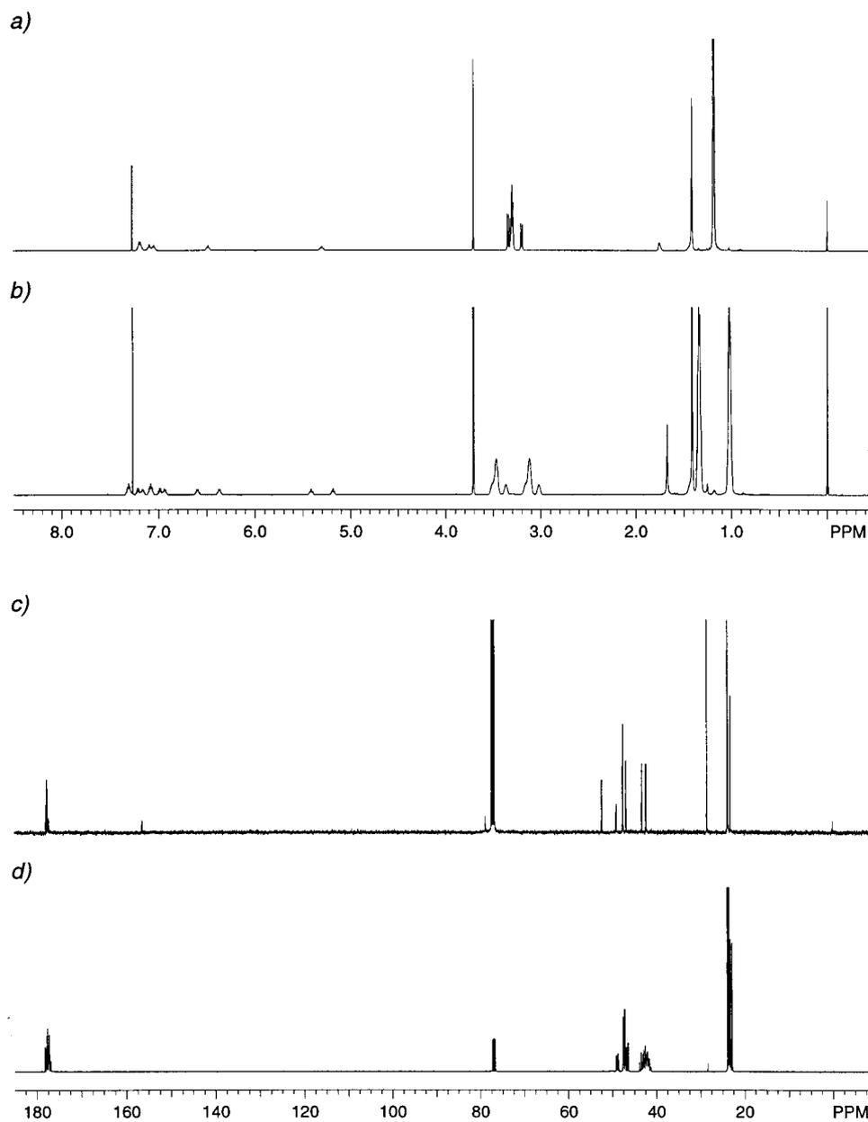
Fig. 3. 400-MHz  $^1\text{H}$ -NMR Spectra of a) the unlabeled hexapeptide **2a** and b) the  $^{13}\text{C},^{15}\text{N}$ -labeled hexapeptide **2a**. 100-MHz  $^{13}\text{C}$ -NMR Spectra of c) the unlabeled hexapeptide **2a**, and d) the  $^{13}\text{C},^{15}\text{N}$ -labeled hexapeptide **2a\***. All spectra were measured in  $\text{CDCl}_3$ .
