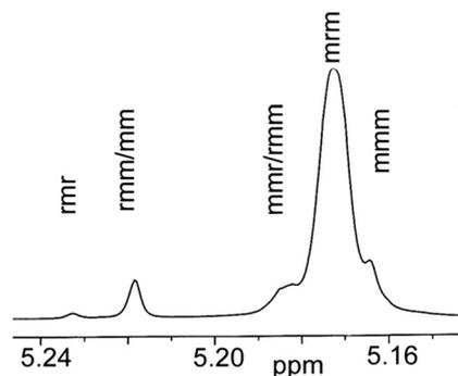
Fig. 4 Homonuclear decoupled  $^1\text{H}$  NMR spectrum of the methine part of poly(*rac*-LA) by complex **2** at  $25^\circ\text{C}$ ,  $P_m = 0.70$ , Table 1, entry 13, 500 MHz,  $\text{CDCl}_3$ .
