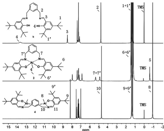
Fig. 2 Stacked figure of the representative  $^1\text{H}$  NMR spectra of pro-ligand **b**, complex **2** and complex **4**.
