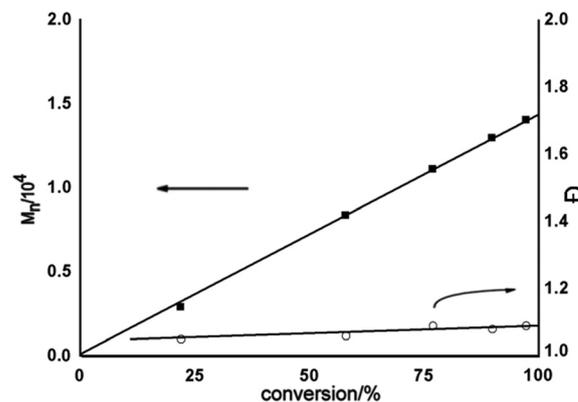
Fig. 6 The relationship between  $M_n$  or  $\bar{D}$  of the polymer and *L*-LA conversion employing complex **2**/isopropanol,  $[\text{LA}]_0/[\text{Al}]_0 = 100$ , at  $70^\circ\text{C}$  in toluene.
