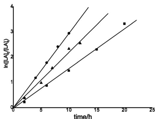
Fig. 5 Kinetics of the ROP of *L*-LA by **2** with isopropanol at  $70^\circ\text{C}$  in toluene with  $[\text{LA}]_0 = 0.5 \text{ mol L}^{-1}$ ;  $k_p = k_{\text{app}}/[\text{Al}]_0$ : ■: *L*-LA,  $[\text{LA}]_0/[\text{Al}]_0 = 100$ ,  $k_{\text{app}} = 0.1703 \text{ h}^{-1}$ ; ▲: *L*-LA,  $[\text{LA}]_0/[\text{Al}]_0 = 75$ ,  $k_{\text{app}} = 0.2280 \text{ h}^{-1}$ ; ●: *L*-LA,  $[\text{LA}]_0/[\text{Al}]_0 = 50$ ,  $k_{\text{app}} = 0.3388 \text{ h}^{-1}$ .
