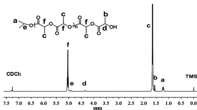
Fig. 8  $^1\text{H}$  NMR spectrum of a polymer sample obtained from the complex **2** system with  $[\text{LA}]_t : [\text{2}]_t = 20 : 1$ .
