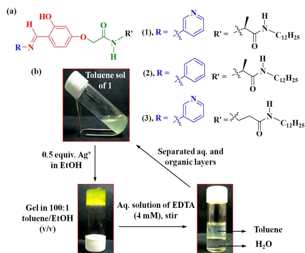
Fig. 1 (a) Molecular structures of the salicylideneanilines ( 1–3 ); (b) photographs showing Ag + -mediated reversible sol-to-gel transition of 1 (3.9 mM) in toluene in presence of 1% EtOH (v/v).
