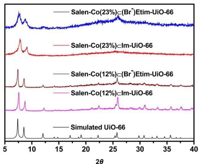
**Fig. 1** PXRD patterns of the simulated UiO-66 (black line), Salen-Co(12%)*c*Im-UiO-66 (purple line), Salen-Co(12%)*c*(Br)<sup>-</sup>Etim-UiO-66 (wine red line), Salen-Co(23%)*c*Im-UiO-66 (red line) and Salen-Co(23%)*c*(Br)<sup>-</sup>Etim-UiO-66 (blue line).
