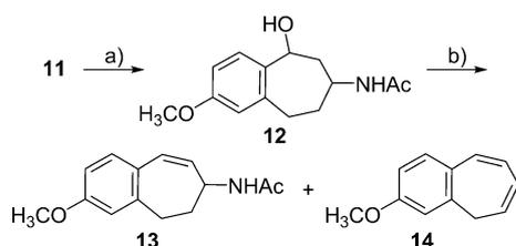
**Scheme 2.** Elimination reactions of hydroxyamide **12**. *Reagents and conditions:* a)  $NaBH_4$ ,  $CH_3OH$ , RT, 16 h, 56%; b) HCl, 5 M, DMF, 60 °C, 24 h, 12% (**13**), 8% (**14**).
