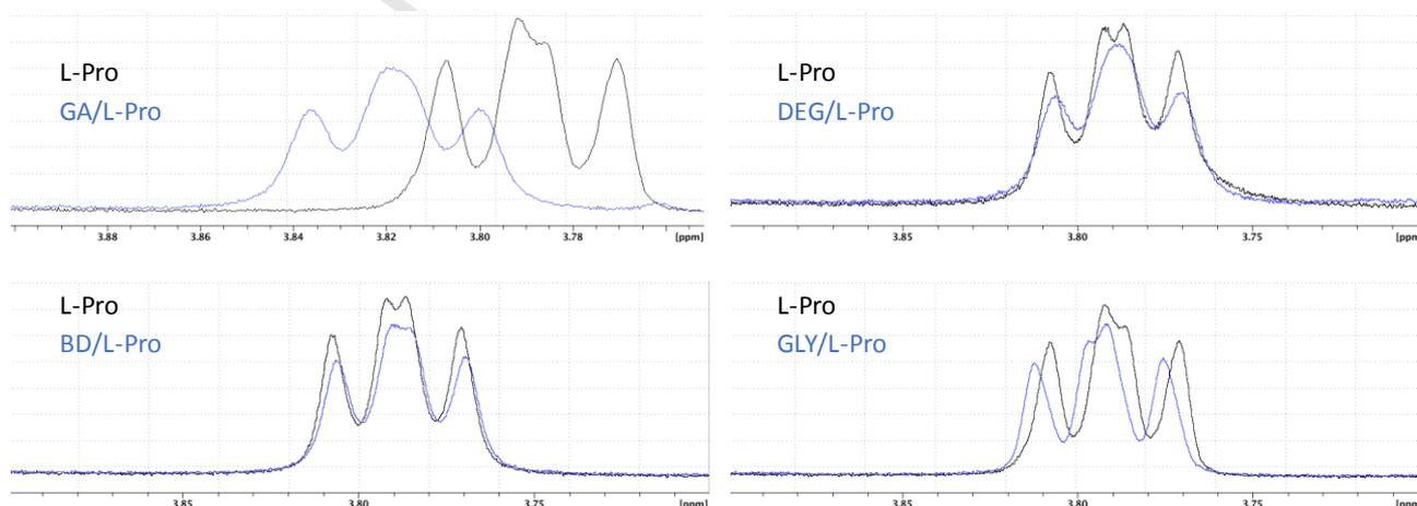
**Figure 1:** <sup>1</sup>H NMR (400 MHz, CDCl<sub>3</sub>/MeOD: 75/25 v/v) spectra of H2 of L-Proline (black) the corresponding CDES (blue).
