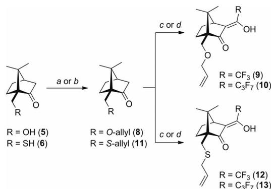
Scheme 2. Allyl/allylthio ether formation and fluoroacylation steps. *Reagents and conditions:* (a) NaH,  $\text{C}_3\text{H}_5\text{Br}$ , THF, 0–50 °C, 2 h, 84% for **8**, 94% for **11**. (b) LiH,  $\text{CF}_3\text{CO}_2\text{Me}$ , THF, 0–67 °C, 14 h, 94% for **9**, 94% for **12**. (c) LiH,  $\text{C}_3\text{F}_7\text{CO}_2\text{Et}$ , THF, 0–67 °C, 14 h, 75% for **10**, 77% for **13**.
