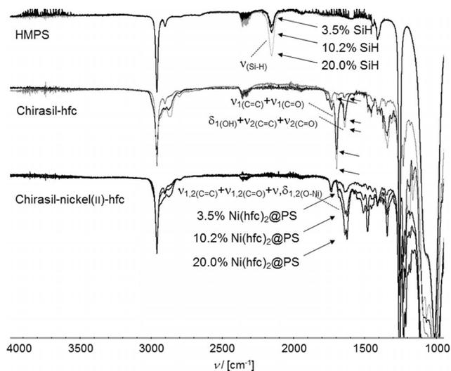
Figure 1. Immobilization of camphor diketone ligand **10** on polysiloxanes (SiH content: 3.5, 10.2, and 20.0%) and nickel(II) incorporation monitored by IR spectroscopic measurements (overlay of nine spectra, characteristic absorption bands marked with arrows): Chirasil-Nickel-OC<sub>3</sub>.
