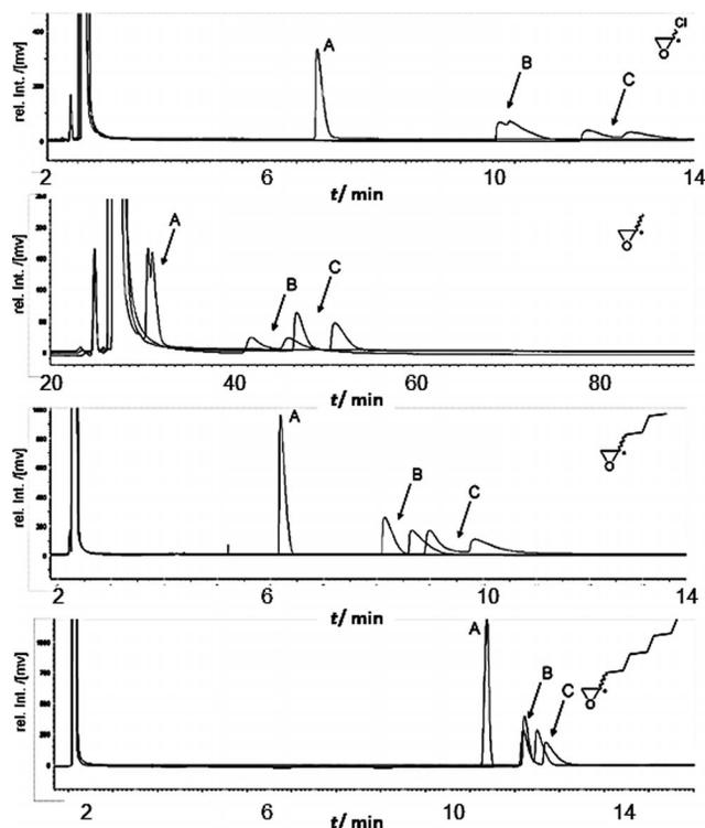
Figure 4. Enantiomer separation of oxiranes using Chiral-Nickel-OC<sub>3</sub> stationary phases with varying selector concentration (a) 3.5% (17), (b) 10.2% (18), and (c) 20.0% (19); enantiomeric pairs highlighted with arrows. Separations were performed using Chiral-Metal-OC<sub>3</sub> coated fused-silica capillaries, 250 nm film thickness; carrier gas: helium; conditions (top to bottom): 50 °C, 85 kPa; 40 °C, 85 kPa; 100 °C, 85 kPa and 110 °C, 120 kPa.
