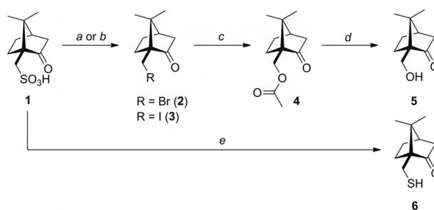
Scheme 1. Routes to 10-hydroxy- (**5**) and 10-thiocamphor (**6**). *Reagents and conditions:* (a) KOH, H<sub>2</sub>O, room temp., quant.; PBr<sub>5</sub>, Et<sub>2</sub>O, 35 °C, 48 h, 35%; (b) I<sub>2</sub>, PPh<sub>3</sub>, toluene, 111 °C, 16 h, 98%. (c) KOAc, HOAc, 175 °C, 12 h, 93% for **2**, 97% for **3**; (d) KOH, MeOH, 65 °C, 6 h, 92%; (e) SOCl<sub>2</sub>, 80 °C, 4 h; PPh<sub>3</sub>, H<sub>2</sub>O, dioxane, 4 h, 100 °C, 94%.
