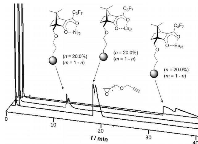
Figure 5. Influence of metal-chelate on the enantioseparation using Ni(hfpc)<sub>2</sub>@PS (19), Eu(hfpc)<sub>3</sub>@PS (23), and La(hfpc)<sub>3</sub>@PS (24); Conditions: 25 m × 0.25 mm i.d., 250 nm film thickness; 80 °C, 85 kPa helium as carrier gas.
