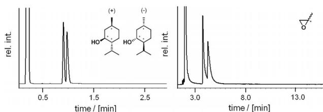
Figure 6. Separation of the enantiomers of (+/–)-menthol and methyloxirane using the novel Chirasil-Nickel-OC<sub>3</sub> CSPs (left: 5 m × 0.25 mm i.d., 500 nm Chirasil-Nickel-OC<sub>3</sub>, 140 °C, 85 kPa; right: 250 nm mixed phase 50% Chirasil-Nickel-OC<sub>3</sub> in GE SE 30, 60 °C, 85 kPa).
