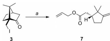
Scheme 3. Regioselective, base-induced camphor cleavage to methylenecyclopentyl ester **7**. *Reagents and conditions:* (a) NaH,  $\text{C}_3\text{H}_5\text{OH}$ , DMF, 80 °C, 24 h, 54%.
